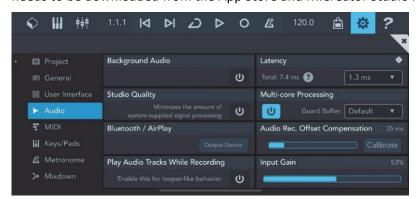
In the audio settings, an "Input Gain" slider can be found with an adjustment range from 0% to 100% - with 0% already muting the signal and 100% representing the maximum additional 15dB. To achieve the minimal gain of 0dB, the slider must be set to 1%.
