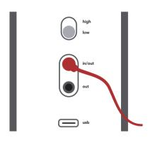
Note: The supplied MCC1 instrument cable includes electronic components in the plug for automatic cable detection (e.g., to automatically switch the plug-in power and the input impedance). Therefore, only use the supplied MCC1 Instrument cable to connect instruments.
