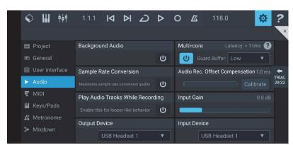
found in the audio settings which allows up to 12dB of gain and -40dB dampening respectively.
