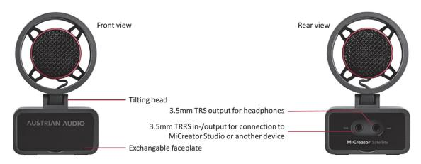
Note: The 3.5mm TRRS jack designated "link" is wired according to the CTIA/headset standard. Since the microphone signal is on pin 4, interference with signal transmission can occur with an unsuitable TRRS cable. Therefore, only use the supplied MCC2 Link cable which has the signal ground and shielding on pin 3.
