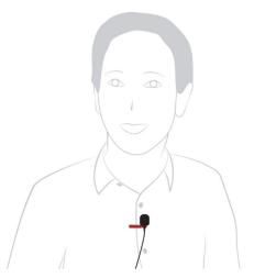
The windshield attached to the microphone also protects against breathing noises and should therefore always be used even when recording in a windless environment, as it does not change the sound.
