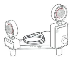
Note: The MCMB MiniBar always guarantees a distance of 17cm between the capsules. This complies with the standard for the ORTF stereo technique defined by the "Office de Radiodiffusion Télévision Française". For the best possible result, the two microphones should be at an opening angle of 110° to each other.
