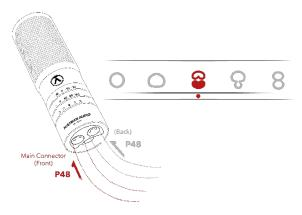
The *OC-S10* will now work in *dual mode*, with the signal from both of the capsule membranes being transmitted independently. In *dual mode*, you may record the two signals to two tracks and use our *PolarDesigner* (or *StereoCreator*) plugins to modify the polar pattern in post-production.
