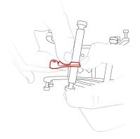
Press the top pad over the bigger top mount point first, then slip it over the two smaller, outer mount points.
